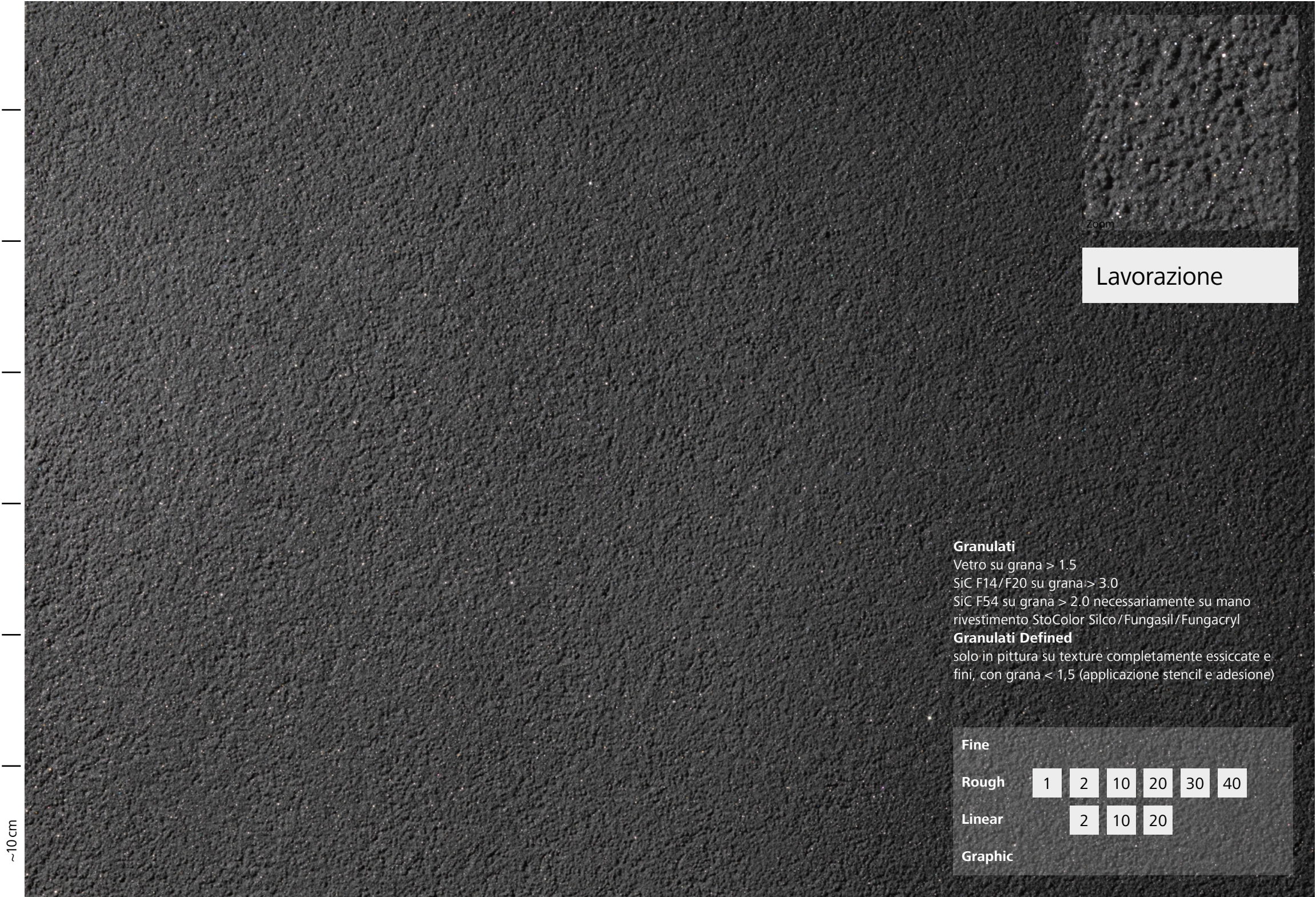
Texture: Rough 1, Stolit K 3.0 (37104) + Effect: Granulate 30, StoColor Fungasil (37104)/Sto-Carburo di silicio F54
